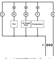
Figure 1: RAK163P1 5-Wire Connection
